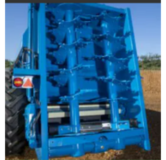
Twin dynamically balanced vertical augers – MK4
