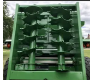
Twin dynamically balanced vertical augers - Widebody
